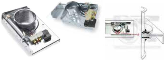
Truly "air-tight" blast gates operate manually or pneumatically and utilize a two part, self-sealing gasket assembly to completely isolate outside air, guaranteeing no air leakage across the valve or into the atmosphere. Designed to withstand 16 Hg" of negative pressure. Available in Zinc Plate or Stainless Steel.
